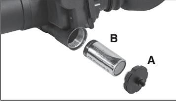
Install standard CR123A batteries as follows:
