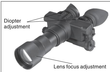
To focus the NVB3X, first you will need to adjust the diopter. Simply turn the diopter clockwise until it stops. Then, while looking through the diopter at an object, slowly turn the diopter back counter clockwise until the grain in the image is sharp.
